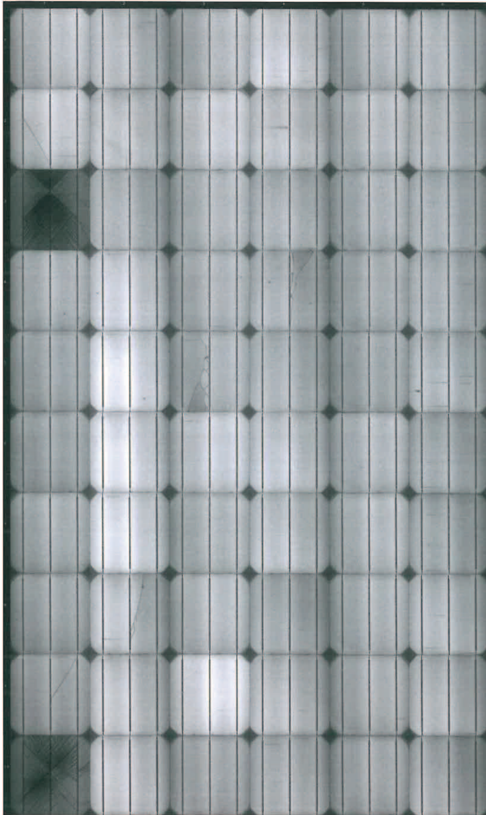
Fig. 11: follow-up electroluminescence image BC 20120005638 tested in combination without the SMB
