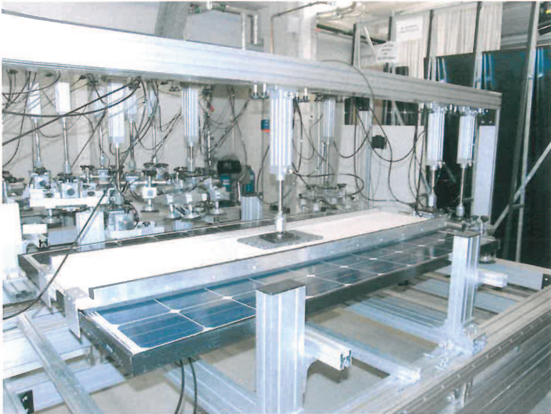
Fig. 5 Test setup 1 st cell in combination with the SMB
