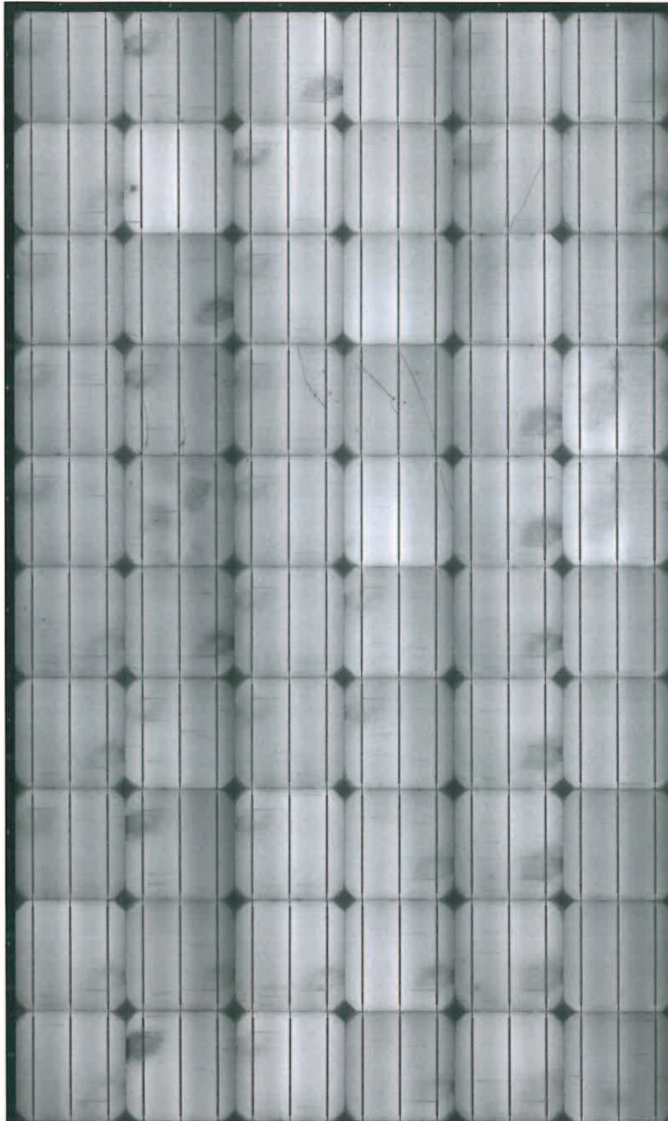
Fig. 9: follow-up electroluminescence image BC 20120005639 tested in combination with the SMB
